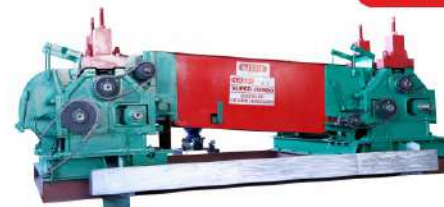
SUPER JUMBO - TOTAL HEAVY - DOUBLE MILL (F.B) WITH PLANETARY GEAR BOX & MOTOR
