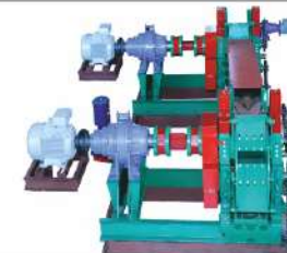
GRAND JUMBO - DOUBLE MILL (F.B) WITH PLANETARY GEAR BOX & MOTOR
